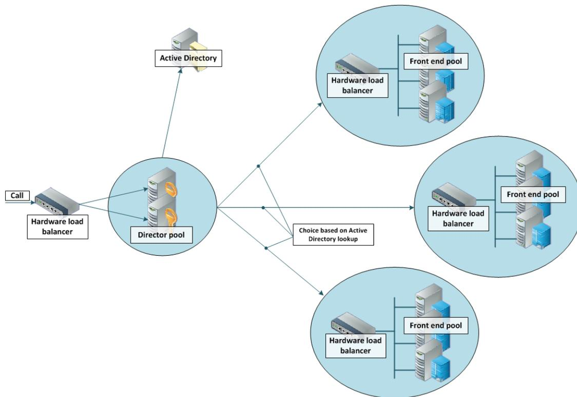
A smaller deployment may not use Lync Director servers, but may just use a Hardware Load Balancer in front of a set of Front End Processors.
