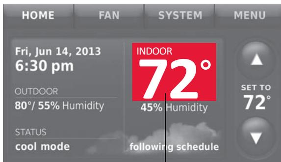
Temperature reading depends on location of sensor
