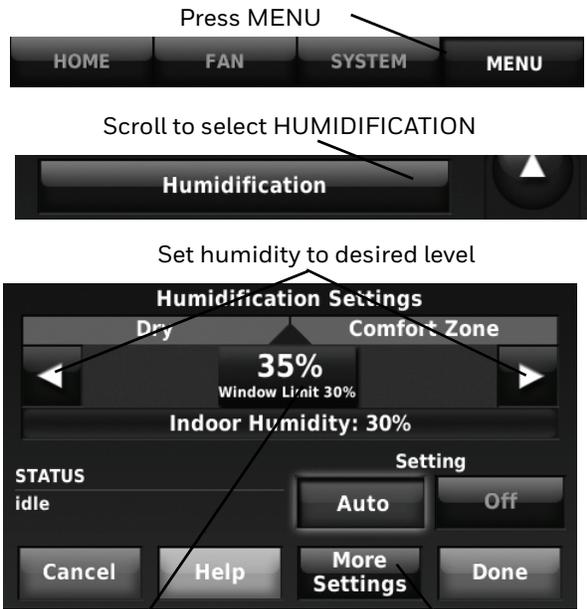
Window Protection limits the amount of humidity to prevent frost or condensation on windows
