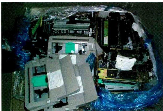
**Figure 2** Some parts vendors purchase used and defective whole unit printers like this pallet-load, then disassemble, test, package, and sell these components. Some companies even warrant and market these parts under the refurbished category. Worn parts like these can cause early failure of a repair and costly callbacks.
