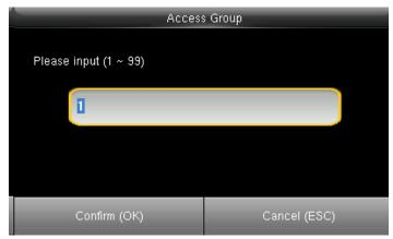
You can change the number for that group in the input section above using the keypad.
