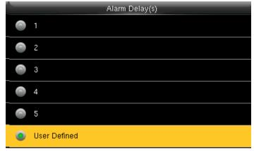
But it can be defined. After some time, alarm signal will be generated automatically. (1-255 seconds)
