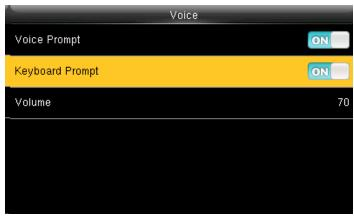
**Keyboard prompt:** This parameter is used to set whether to generate beep sound in response to every keyboard touch. Select ON to enable the beep sound, and select OFF to mute
