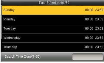
Use numeric keys to search for a time period in the range from 1 to 50. Press ▼ to select the item to be set and press OK
