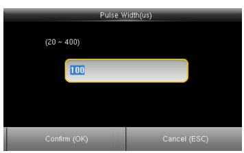
Here you can edit the Pulse width by using the keypad on the clock. The Pulse Width ranges from 20 to 400 (us).
