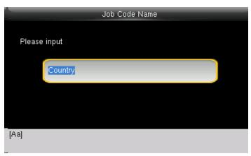
To change the job group name to country as shown above we need to press\* key to switch the input method and type country using the keypad. After that press confirmOK button.
