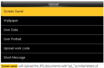
Screen saver will Upload the JPG documents with "ad\_" as initial letters of document names stored in a USB disk to the terminal. After the upload, these pictures can be displayed on the initial interface of the terminal.
