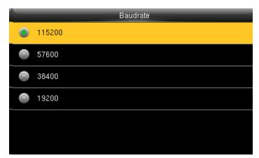
There are five options: 9600, 19200, 38400, 57600 and 115200. If the communication speed is high, RS232 is recommended. If the communication speed is low, RS 485 is recommended
