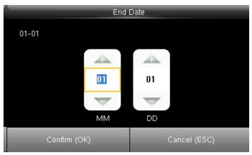
Press / to select a time option and press  $\checkmark$  /  $\blacktriangle$  to set time. After setting a period of time, press  $\bigcirc$ K to save the setting and exit
