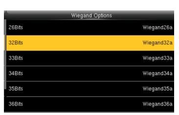
To select 32 bits Wiegand format click on 32 Bits and press OK.
