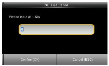
You can change the time period in the input section with the help of the keypad.
