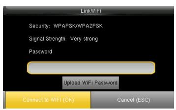
You can select any wireless network you wish to connect and you can upload the password via "USB" or by using the keypad on the clock. Once you upload the password you can press "Connect to WFI(OK)" and the following network will get connected. See NOTE below
