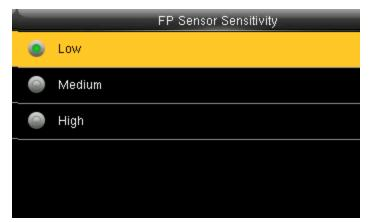
The default value Medium is recommended. You can set the sensitivity of fingerprint collection to High when the response to finger scan lags in a dry environment. When the usage environment is humid, you can set the sensitivity of fingerprint collection to Low if the fingerprint is difficult to identify.
