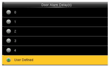
You can set the timing for door to remain open from the options above. The Door Alarm Delay ranges in seconds.
