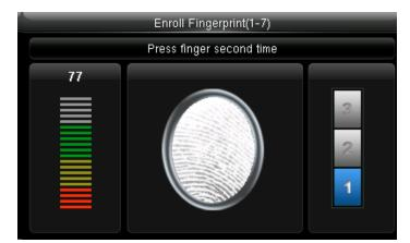
Place the same finger on the fingerprint sensor for the second time.
