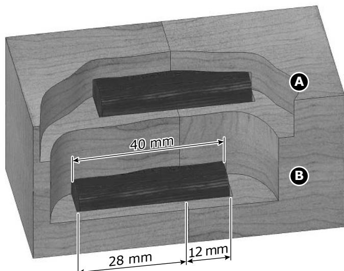
In most cases, the tenon should be centered across the joint, and the depth of the mortise should be  $\frac{1}{2}$  the length of the tenon. However, in some cases you may want to have more of the tenon in one piece than the other.
