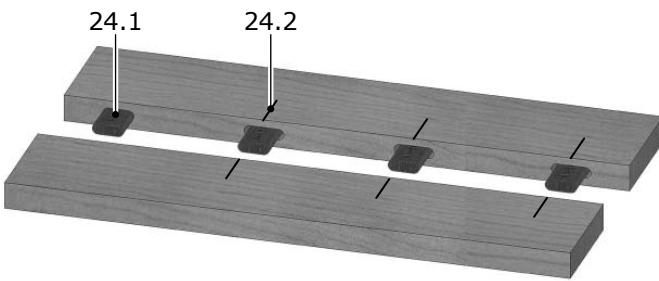
For edge joining boards, a series of tenons are placed down the length of the joint. The first tenon [24.1] is used to register the two boards horizontally, so it is milled at standard width. The remaining tenons align the boards flush and may be milled with an oversize width.
