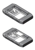
4. Lower the SIM card holder and slide it to the locked position.
